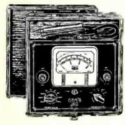
\* AC-DC multi-range nieter using rotary range selectors. Ranges chosen so that commonly measured values fall on upper section of meter scale. Ranges—AC and DC volts 0/3/15/30/-150/300/600—DC at 20,000 ohms per volt—AC at 2,000 ohms per volt. DC mils 0/30/300/3M. Resistance ranges 0/500/50M/20meg with self-contained battery. Model 320—net \$38.50. Triumph Mfg. Co., 4017 W. Lake St., Chicago, Ill.—Selling Sound.
