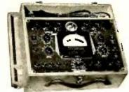
★ Tube tester with floating filament selector. Five tests possible inter-element leakage, open element in each circuit, short check between any 2 elements, quality test of complete tube elements, separate sectional test of dual purpose tubes. Model 501 il-
